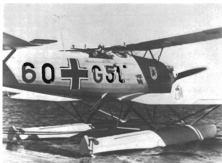
BELOW: The pilot of this Heinkel He 60 C-1, coded 60+G51, of 1./Kü.Fl.Gr 506 has just started his engine and is preparing to move off – however note the mooring line still attached to the central bracing strut on the floats.
