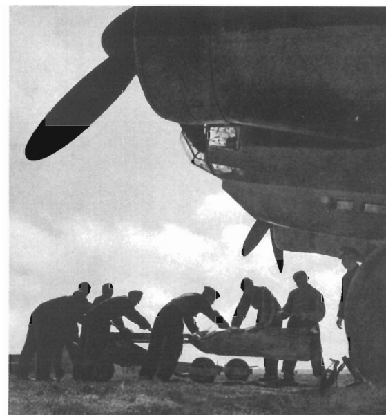
BELOW: Ground crew prepare to load a SC250 bomb from a purpose-built hydraulic trolley into a Ju 88 of KG 30, probably France 1940.
