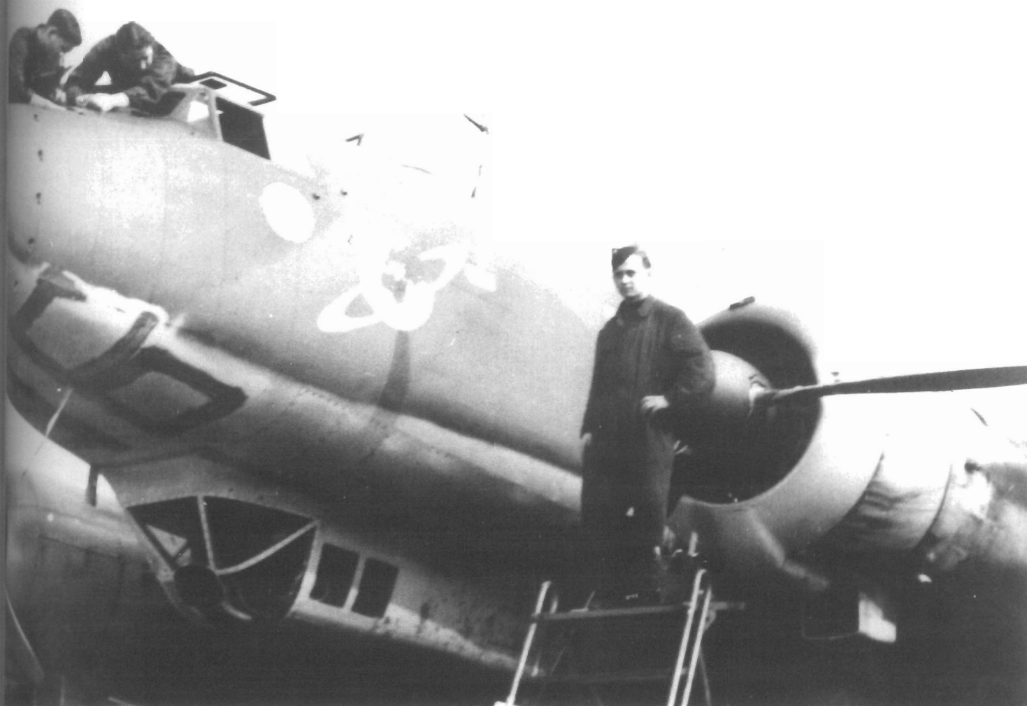
ABOVE: A Focke-Wulf Fw 200 Condor of I./KG 40 in the process of being serviced in either France or Norway in 1940/41. Note the feathered propeller, lack of armament in the ventral gondola, removed for servicing, and the red oxide primer applied roughly to panel joints under the nose.
