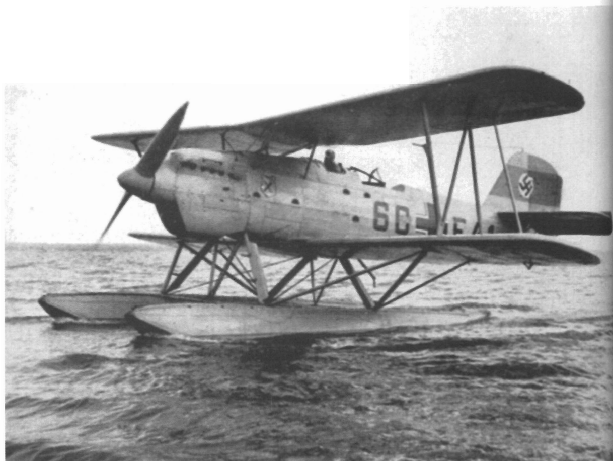
ABOVE: A Heinkel He 59 B-2 coded 60+A13 of 3./Kü.Fl.Gr 106 sits on its beaching trolley at List in 1936. The unit code of '60' was changed in May 1939 to 'M2'. Note the distinctive large radio loop common to the type and the fact that the armament has been removed.
