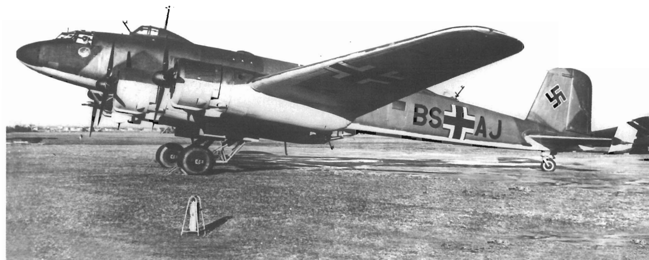
ABOVE: Focke-Wulf Fw 200 Condor C-1, W.Nr.0005, BS+AJ, was built in 1940 but survived only a few weeks before being destroyed during experiments at the Erprobungsstelle Tarnowitz on 21 March that year. The C-1 featured a faired, fixed upper streamlined, blister which was to be the second of a number of progressive design changes for this defensive position.
