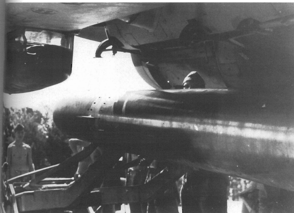
LEFT: To assist Luftwaffe mechanics load heavy torpedoes aboard the racks of its aircraft, in this case a Ju 88, special hydraulic trucks were used.
