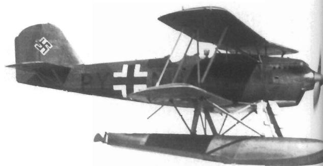
ABOVE: This He 60 D-1 has been re-painted in the Luftwaffe splinter pattern camouflage of the two green RLM 70/71 on the upper surfaces and light blue 65 underneath. The machine still carries the factory radio call sign PY+NW, in black
