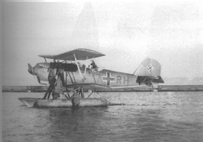
ABOVE: This He 60 coded possibly N7+RH of Seenotstaffel 2, has just landed and is being boarded by mechanics who have made their way to the aircraft in a rubber dinghy. The fuselage Balkenkreuz is of the early war type, having narrow white angles with a thin black outline. The aircraft is painted in a RLM 71/72 splinter pattern with 65 beneath.
