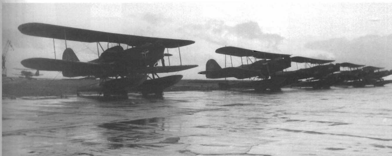
ABOVE: Taken on 26 October 1939 at Wilhelmshaven, these five canvas-covered Heinkel He 59 Bs from 3./Kü.Fl.Gr 406 stand ready on their beaching trolleys waiting for a break in the inclement weather. Another aircraft can be seen in the distance beneath the crane. All the aircraft in the foreground carry the white winged sword on a black shield emblem of 3./Kü.Fl.Gr 406. This emblem was adopted by 3./Kü.Fl.Gr 506 shortly after this photograph was taken.
