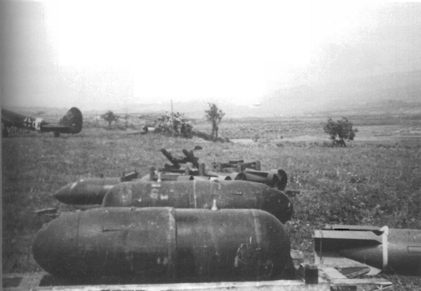
ABOVE: A Junkers Ju 88 of III./KG 30 stands by between operations. In amongst the ordnance in the foreground lie some Luftmine A (LMA) aerial mines. A smaller version of its larger brother the Luftmine B and using the same form of deployment, it weighed in at 500 kg and measured 1.8m in length.
