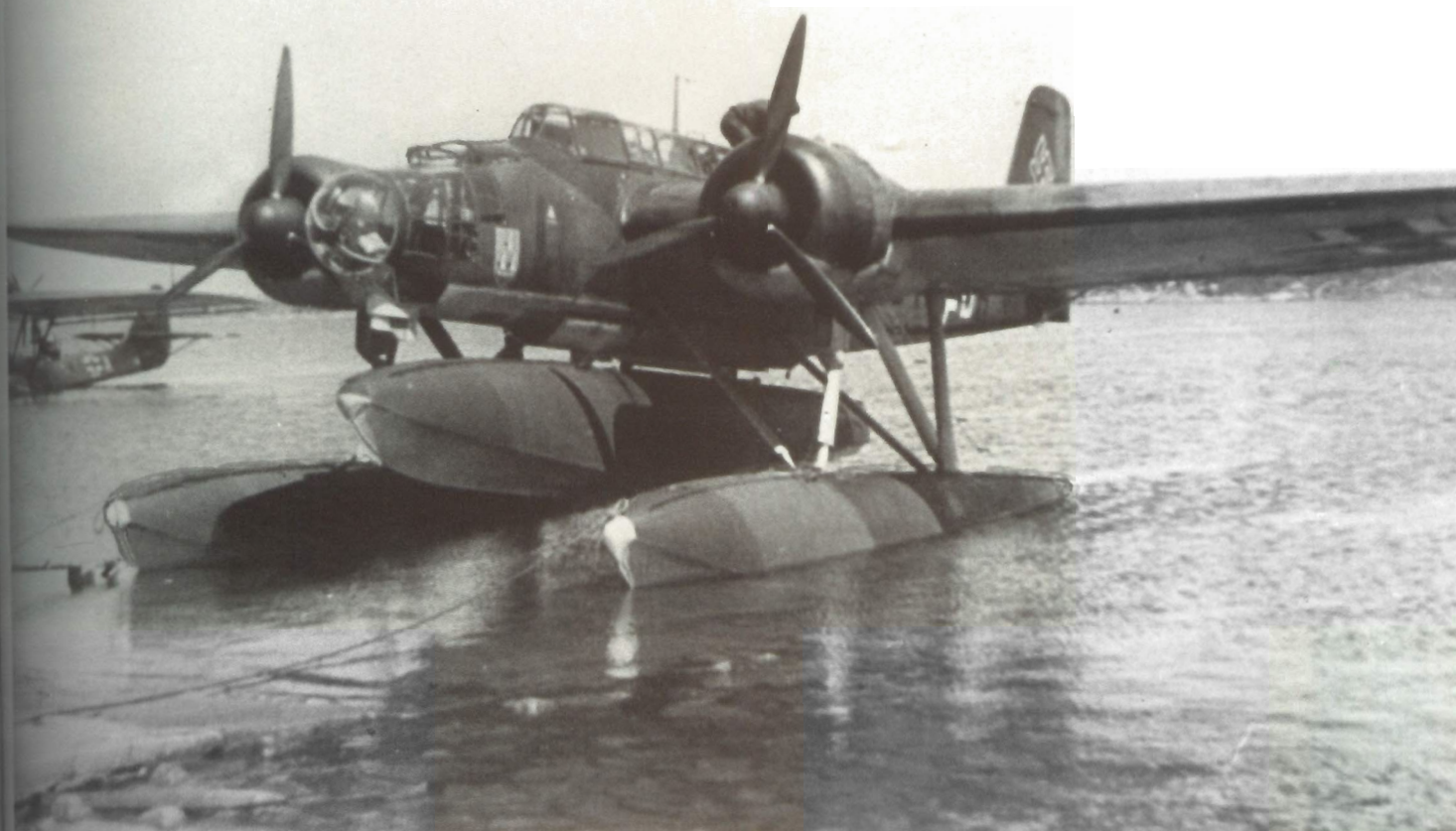
ABOVE: Due to the choppy sea conditions and the risk of surface debris and rocks, floatplanes often suffered damage to their floats necessitating repairs or complete replacement. Here a He 115 C from 1./Kü.Fl.Gr 506 has been fitted with a spare float ready for delivery to one of the many bases along the Baltic Coast in 1939 or 1940. The aircraft carries the Staffel shield-shaped emblem of three oystercatchers flying against a blue sky above the waves.
